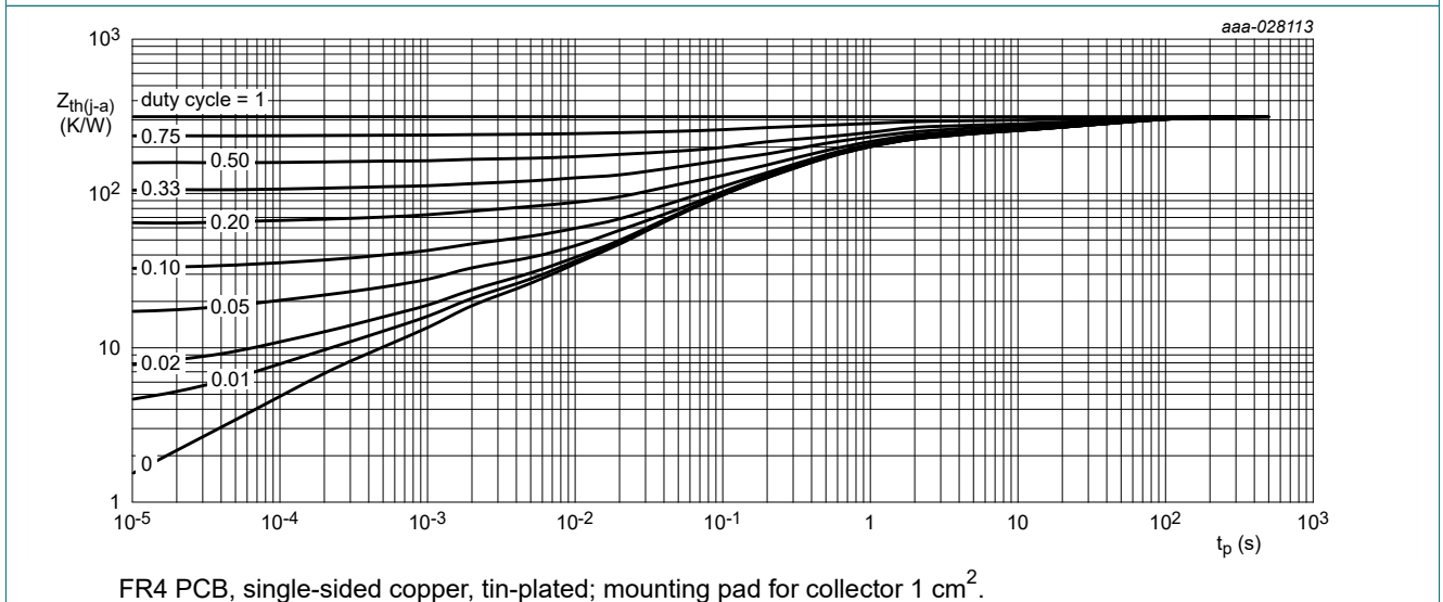
Fig. 3. Transient thermal impedance from junction to ambient as a function of pulse duration; typical values
