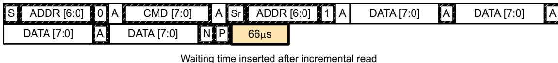
Figure 8. I 2 C Command Wait Time
