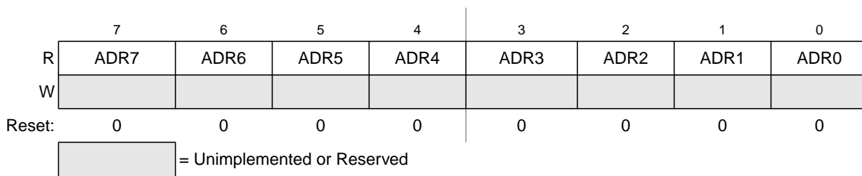
Figure 9-7. Data Result Low Register (ADCRL)
