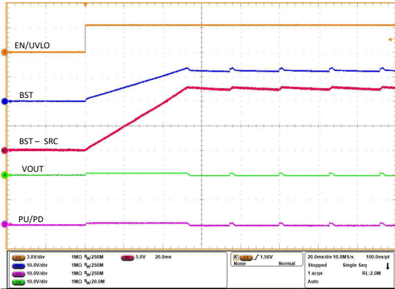
Figure 9-2. Start-Up Profile of Bootstrap Voltage for INP = GND and C_{BST} = 470 \text{ nF}
